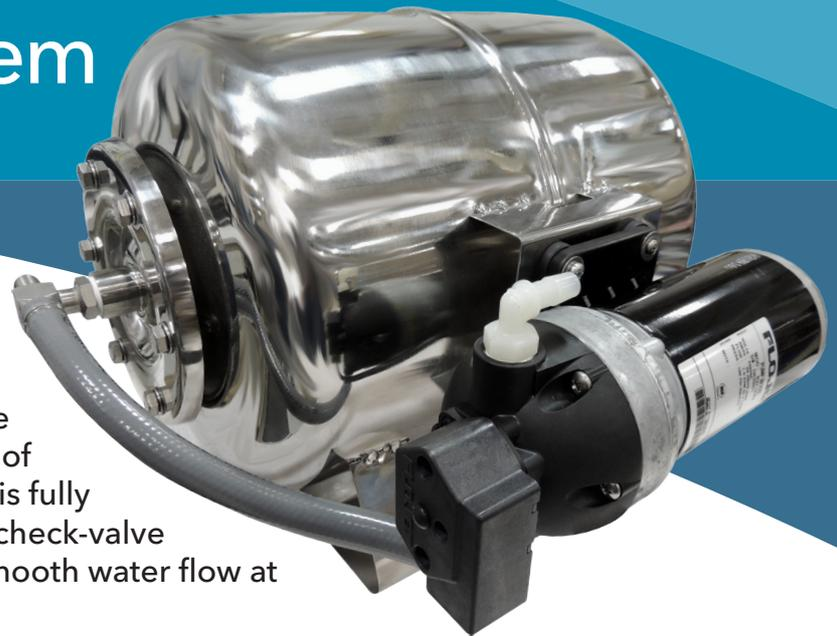
FLOJET 2 Gallon SS Water Booster System is designed to provide a constant water pressure of up to 87 psi (6 bar) and a maximum flow rate of 1.5 gpm (5.7 lpm) at 10 psi (0.7 bar). The pump is fully automatic, with an integral pressure switch and check-valve to maintain system pressure and will supply a smooth water flow at various requirement levels.
